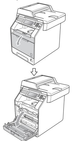
8 Hold the green handle of the drum unit. Pull the drum unit out until it stops.
